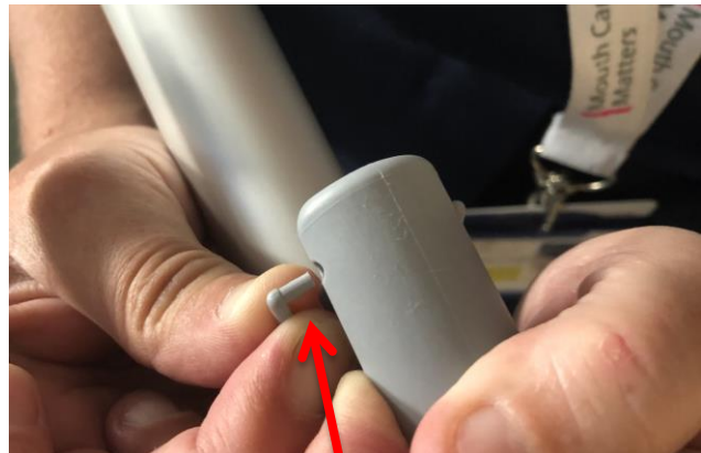
If the safety clip pin detaches and 'pings off'. Do not use, label 'out of order'. Complete an incident report (Datix). Report to Hillrom.
