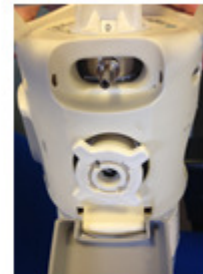
Pull down grey flap, attach oxygen and select the flow rate (if using the firtree outlet)
